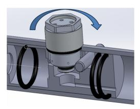
It is important that during the mounting of the regulator you go slowly so you have a feel for the orings seating in their recesses. Also when fully seated you will need to apply a little torque so the regulator is completely seated and the small nozzle in the regulator is held firmly in its place and has no play.
