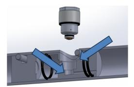
Then screw in the regulator using a 19mm Hex socket.
