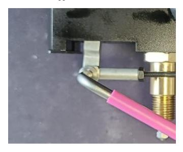
The whole rail/shroud assembly can now be slid of the barrel and tube. As well as the plastic cover behind the picatinny.
