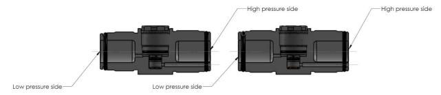
The correct orientation can be seen above, the side with the smaller hole underneath the big central hole is the high pressure side. The one with only a larger center hole is the low pressure side.
