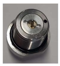
A 5 minutes turn counter clockwise will give a pressure increase of about 4-5 bar. Or ca 25-30 bar for  $\frac{1}{2}$  a turn
