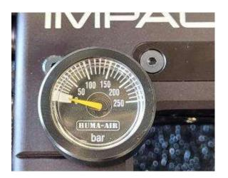
The new gauge will indicate the first stage regulator pressure.
