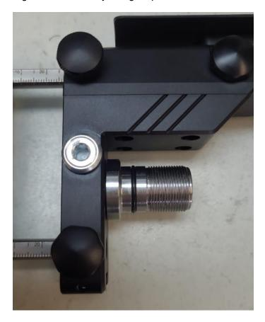
Now put some silicone on the orings on the regulator and inside the colar and mount the colar over the regulator. The gauge can be oriented both left and right. So choose what is most convenient for you.
