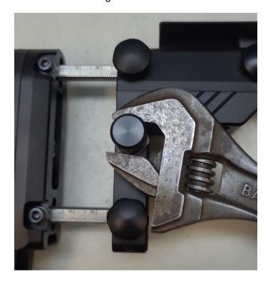
Take your collar from the bag and screw in the fill foster into the hole that has a small slot on the bottom. The locating tab is also on this side of the colar.
