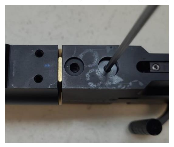
Now remove the actual valve from the regulator housing using a spanner. To push out the regulator afterwards you can point the opening that shows the original regulator in a pile of towels to catch the reg and carefully screw on the bottle. This will push out the regulator. And the pile of towels avoids any damage. The parts layed down in order will look like this.
