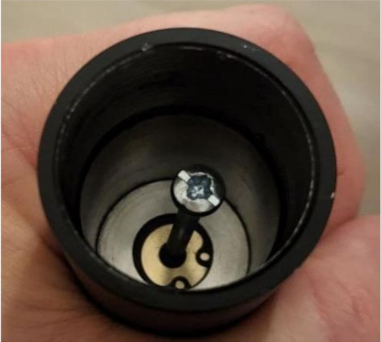
Optionally you can heat the tube up with a hairdryer around the area where the regulator is fitted in the tube to loosen up stuck grease. Now gently but with a firm hand pull the regulator out of the tube. It'll take some force to get it going.
