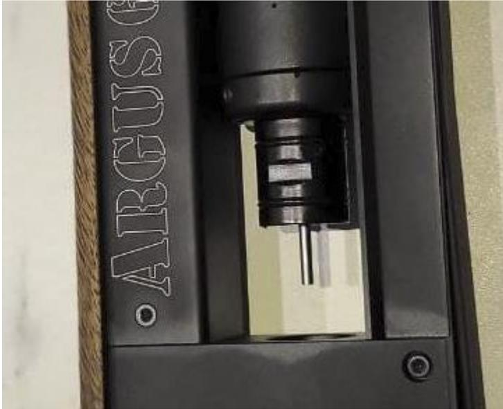
Before you re-install the cylinder completely into the action you need to slide the small spring onto the valve stem and then gently push the cylinder all the way into the action taking care not to damage the orings on the valve body.
