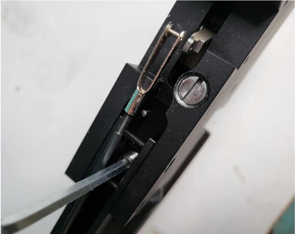
You could also remove the trigger linkage that goes back to the action and actuates the shear to make it easier to access this set screw, to do that just spread the two legs so the linkage can slide out of the captive hole as indicated below.
