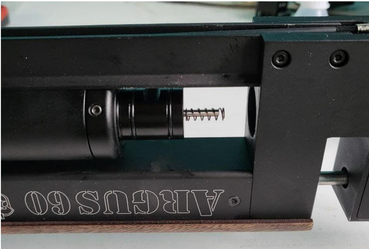
Now tighten the large setscrew and tighten the 4 screws on each side. Do not over torque these screws.
